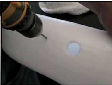
Drill a 5/32" hole at your mark for the attachment of the lock.
